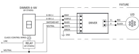
DIML2 0-10V DIMMING W/RELAY TO SWITCH POWER
