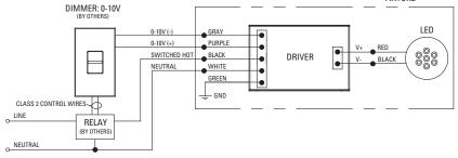
DIML6A, 6B 0-10V DIMMING (NO RELAY)
